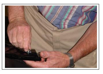
g. Install the lift the dot stud, washer and nut on both the drivers and passenger's side of the car.
