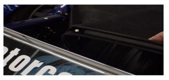
**f.** You will need to cut a small slit inside of the header bow to allow the pin in the center of the bow to come through the fabric. This picture shows the fabric wrapped and also weather-strip inserted inside the channel, you may do this to help the top seal tighter to the windshield if you wish.
