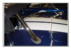
**r.** Mark the locations of the remaining 8 lift the dot studs in the body. This location is based on the tape mark you put down in the previous step for the correct front to back spacing. We usually space them approximately 7 inches apart left to right. Be sure to follow the location of the top, and be careful that your spacing does not interfere with your roll bar bezels or anything else that might be on your car. Drill and install the 8 remaining studs.
