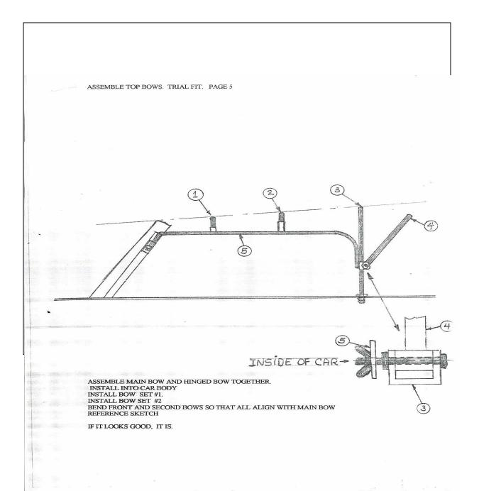
Install the 3/8 ID rubber piece K onto piece 5 as labled in the above diagram, this will hold the metal support off of the inside of the windshield frame. You will need to lubricate the rubber to slide it into place.
