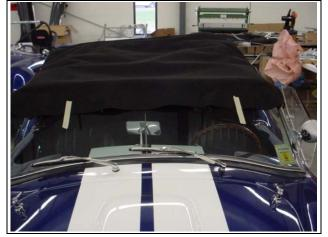
**g.** Pull the top into position; line up the sides of the top behind the doors. Locate the front of the sewn flange of the top even with the back of the doorjamb on both sides of the car. This photo shows the lift the dot installed so you can see the correct location of the snap.
