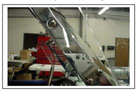
b. 1.250" below these 2 holes, and ¼ inch behind the windshield glass drill a 3/16 diameter hole for the aluminum windshield support tube. If you are using wind wings you may typically use the upper wind wing mounting bracket hole to hold these support tubes.
