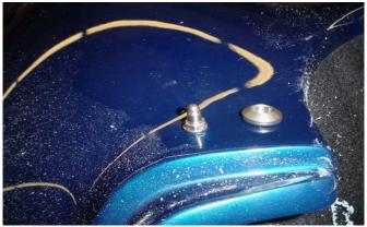
h. Measure 2.875" from inside lip of trunk towards the back of the cockpit, and the center of the trunk measured between the trunk hinges. Drill a 1/8 hole here and install the center rear lift the dot stud.
