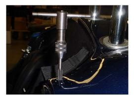
f. Install the o-ring on the ferrule and screw the ferrule into the body. As the ferrule is about 1/2 way down into the body place the 1/2-20 nut under the ferrule and begin screwing the nut onto the ferrule.
