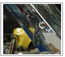
If you have wind wings you will need to reverse the mounting clamps so that the windwings pivot forward so you may open the door with the side curtains installed.
