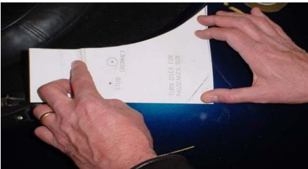
Locate the template on the driver's side and mark the 29/64" hole for the  $\frac{1}{2}$ -20 tap, and the 1/8 hole for the lift the dot stud. Turn the template over and repeat for the passenger side
