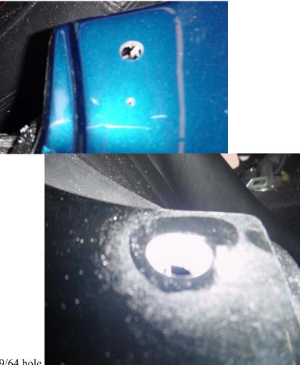
d. Chamfer the 29/64 hole Chamfer the holes when you drill in the door as well.
